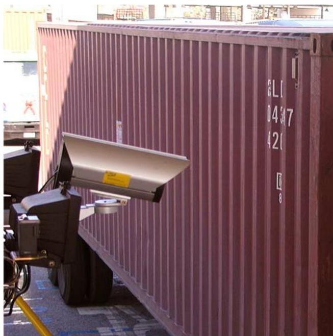
The following photo shows the front view, where a double set of camera/illumination units are used to capture the truck plate:
