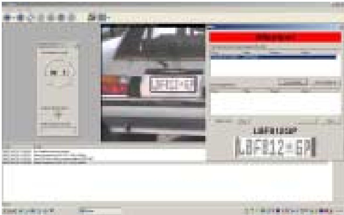
Figure 28 Rear LPR capture and recognition with alarm
