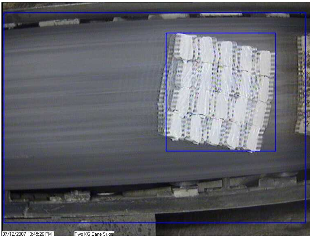
Figure 22 - Two one KG pre-packs were incorrectly classified as two KG Pre-Packs
