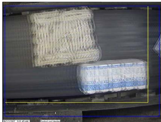
Figure 9 - 1 KG poly bag was touching a 2 KG product. This was manually classified.
