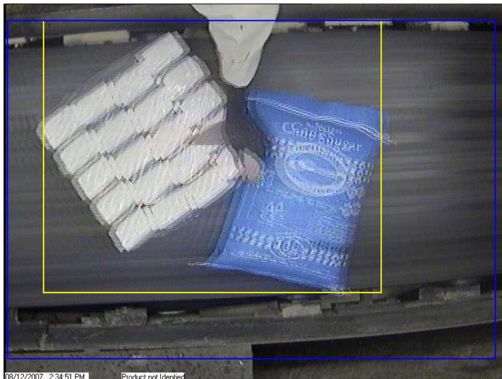
Figure 21 - Bags which cannot be classified due to human interference
