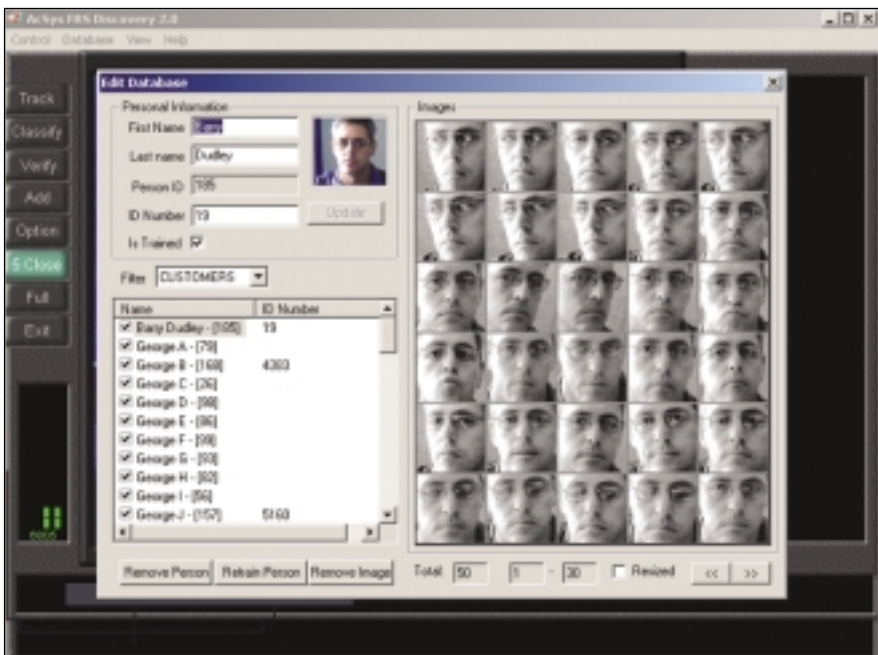
The database screen showing the effect of using a HNET neural network where images with different expressions, at different head angles, lighting conditions and at varying distances from the camera are collected and updated over time.
