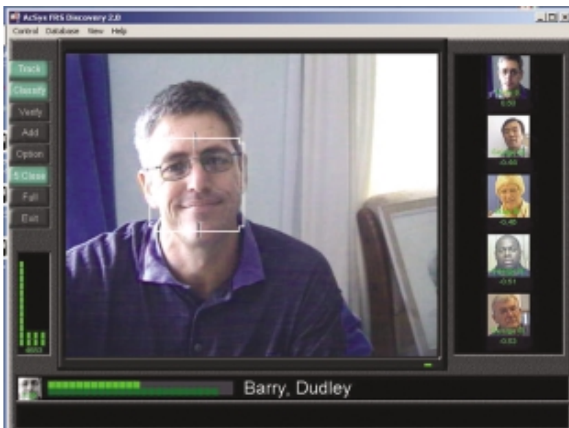
Facial recognition in classification mode (one-to-many identification), with the closest matches displayed on the right side of the screen in descending order of recognition confidence.
