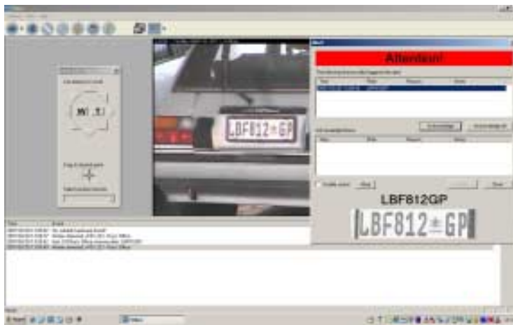
Figure 13 Rear LPR capture and recognition with alarm
