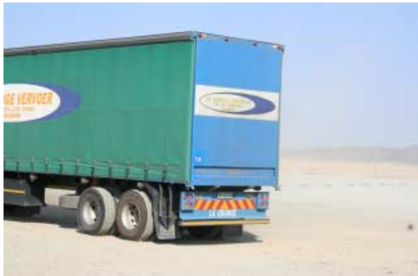
Figure 10 With no front plate present a Rear camera could provide valuable information
